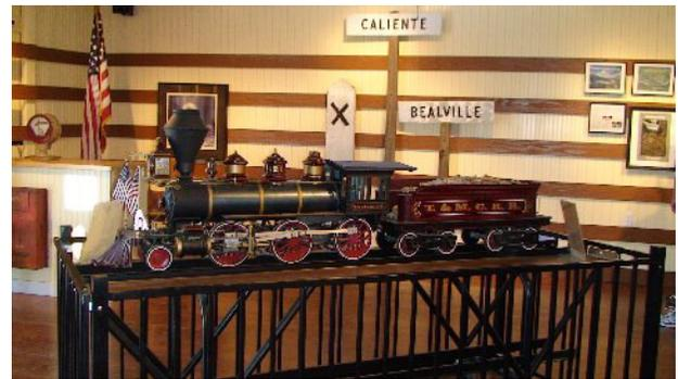
1-1/2" Scale (7" gauge) live steam 2-6-0 "Mogul" type steam locomotive. The Mogul appears to have been constructed from either a Harper Locomotive Works or Little Engines mogul kit. Photo by Elliott Alper
